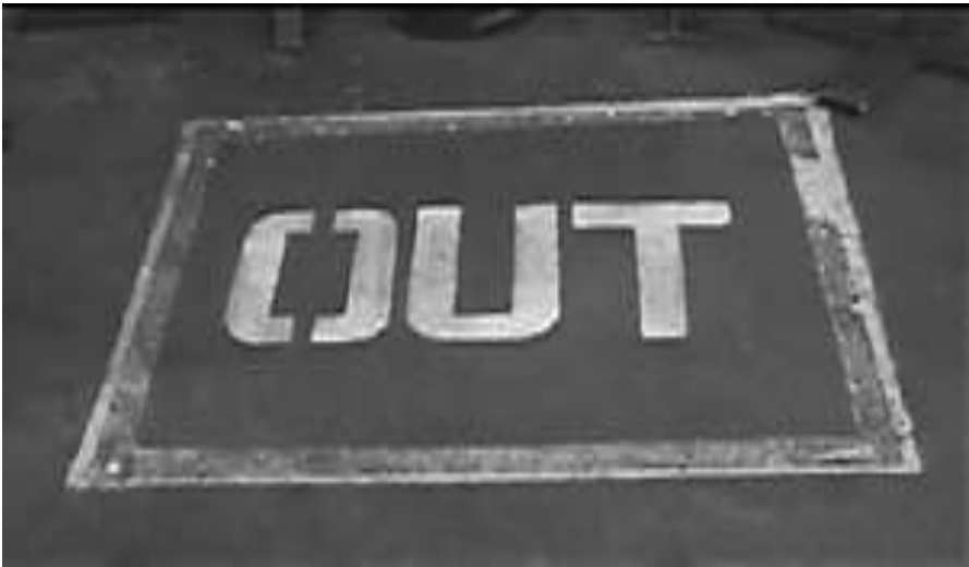
Figure 5-24: Example of a kanban signaling device – the OUT square.
