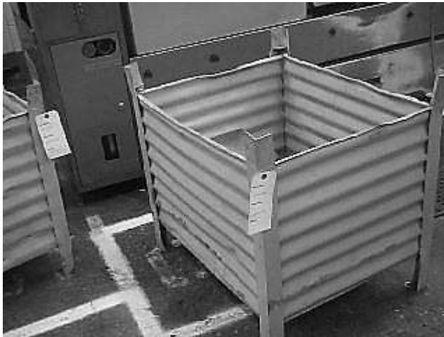
Figure 5-20: CTD Co. uses tote boxes to transfer parts between operations.
