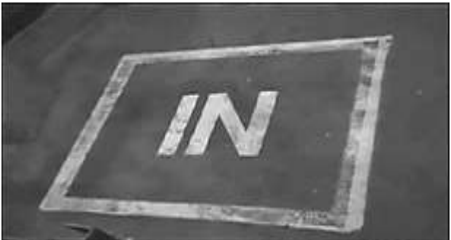
Figure 5-23: Example of a kanban signaling device – the IN square.
