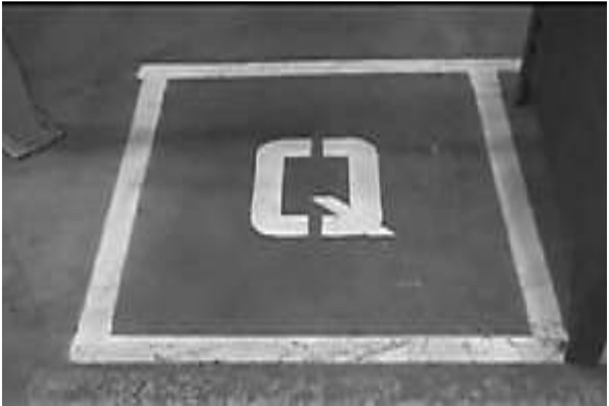
Figure 5-22: Example of a Kanban signaling device – the QUEUE square.
